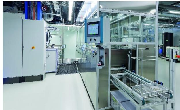
The final cleaning system delivers the product directly into the cleanroom. The system and its conveyor unit are fully enclosed all the way into the cleanroom.
