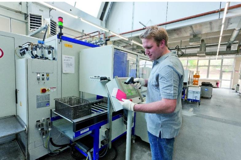
Following the diverse processing steps such as machining, grinding and coating, the parts undergo cleaning in solvent-based systems. The specific cleaning program is selected via bar codes.
