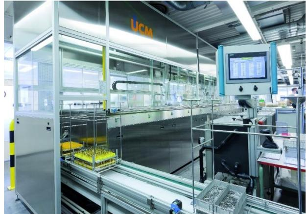
The equipment controller stores 16 different programs for final cleaning of the diverse parts.
