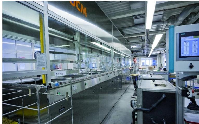
The first stage of the ultrasonic cleaning system used for final cleaning has three separate tanks. Parts consisting of different materials can thus be cleaned separately.
