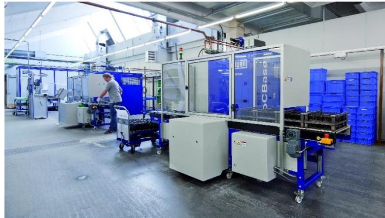
Multiple solvent-based systems are used at the pre-cleaning level in order to separate material flows and to prevent cross-contamination.
